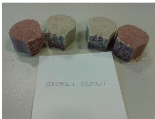
Fig. 5c. Fracture of tensile test specimens - after 24h – of the system: Geopol + Rezolit
