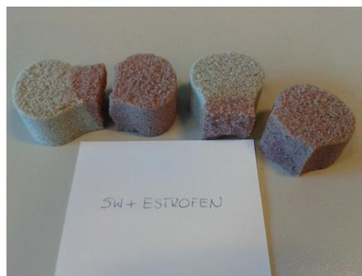
Fig. 5f. Fracture of tensile test specimens of the system: water-glass + Estrofen, after 24h
