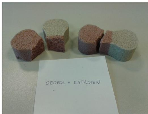
Fig. 5d. Fracture of tensile test specimens – after 24h – for the system: Geopol + Estrofen
