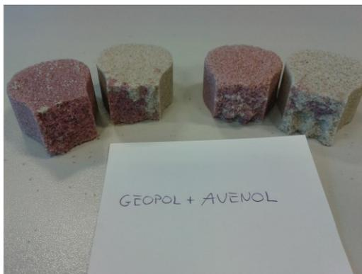
Fig. 5a. Fracture of tensile test specimens - after 24 h - of the system: Geopol + Avenol
