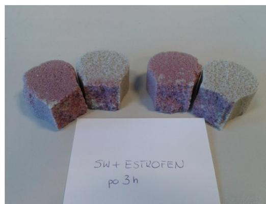
Fig. 5e. Fracture of tensile test specimens of the system: water-glass + Estrofen, after 3h
