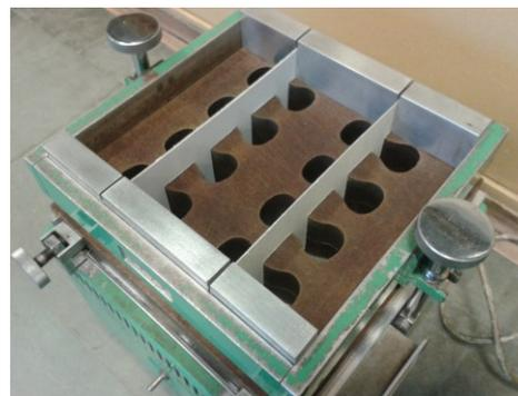
Fig. 2. The way of mounting the partition separating two sands in the LUZ apparatus
