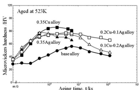
Fig. 1. Age-hardening curves of alloys aged at 523 K
