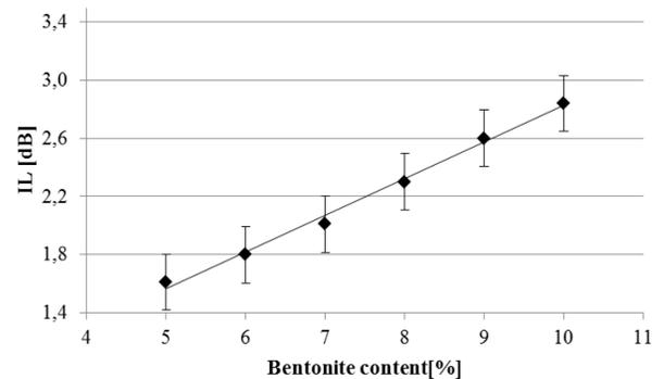
Fig. 5. Effect of bentonite Geco content in traditional moulding sand on insertion losses  $I_L$
