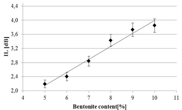
Fig. 3. Effect of bentonite Specjal content in traditional moulding sand on insertion losses  $I_L$
