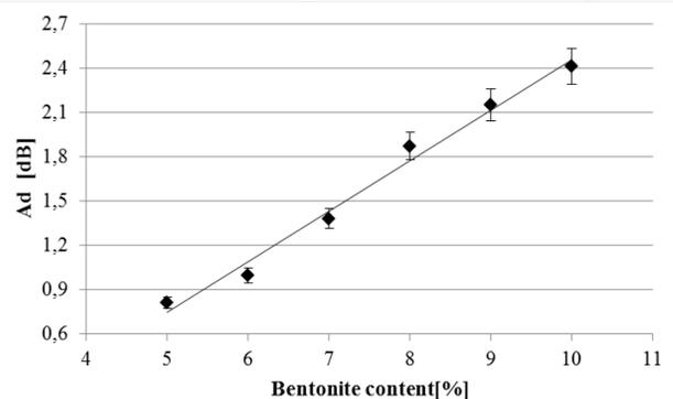
Fig. 4. Effect of bentonite Specjal content in traditional moulding sand on absorption damping  $A_d$
