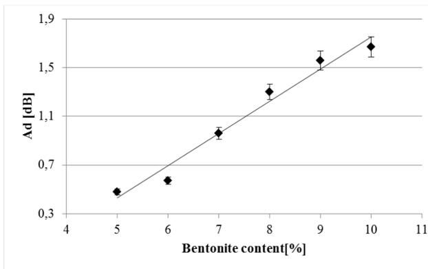
Fig. 6. Effect of bentonite Geco content in traditional moulding sand on absorption damping  $A_d$
