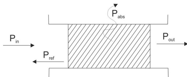
Fig. 2. Balance of microwave power affecting the specimen
