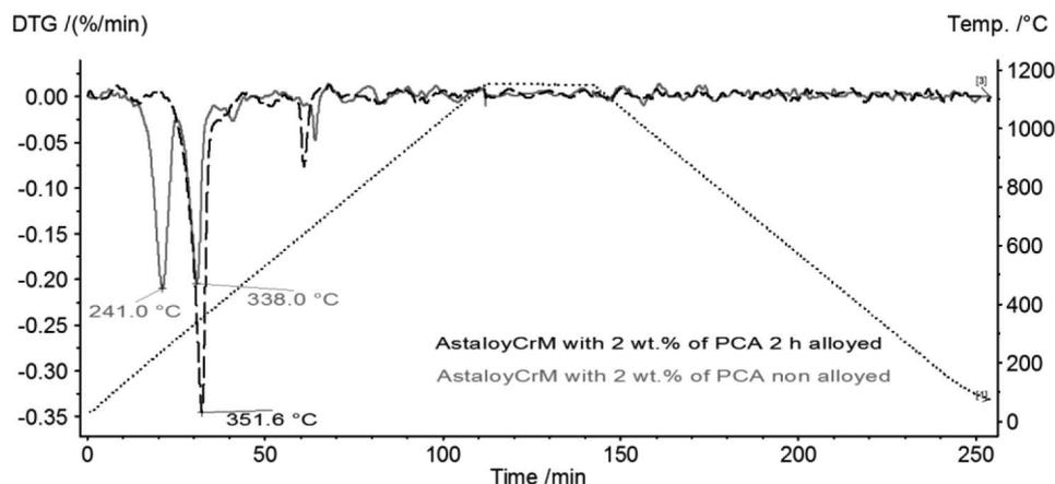
Fig. 9. DTG curves of Astaloy CrM with 2 wt.% PCA, 2 h alloyed and non-alloyed sintered in a helium atmosphere
