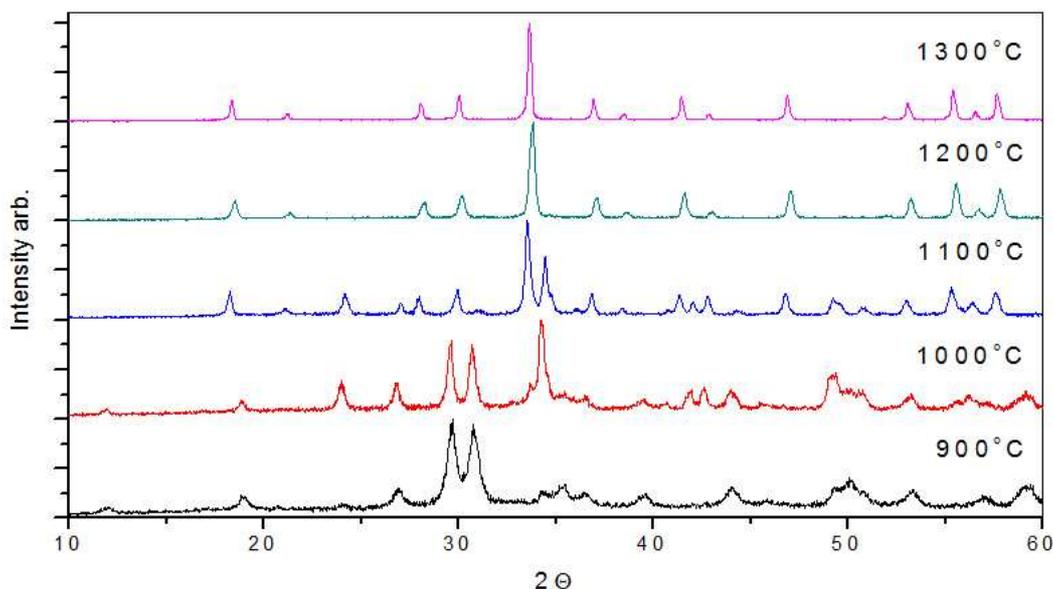
Fig. 1. XRD patterns of the YAG:Ce samples calcined at 900°C(a); 1000°C(b); 1100°C(c);1200°C(d); 1300°C(e) for 1h
