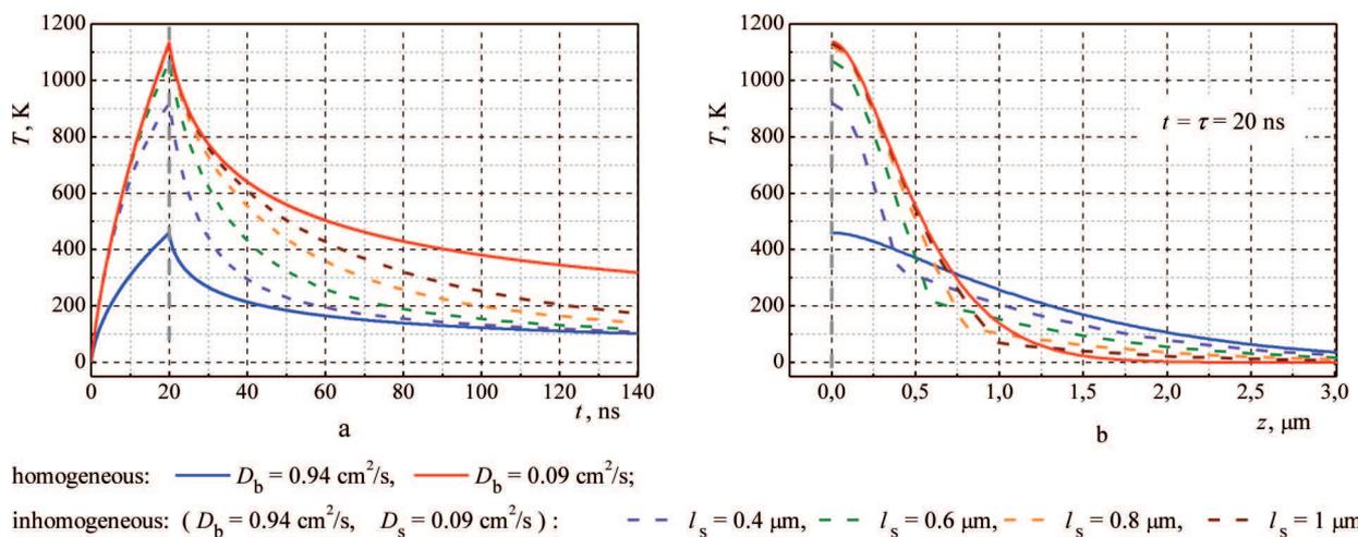
Fig. 4. Surface temperature evolution (a) and temperature profiles (b) at the end of laser pulse for model two layer structures with different thickness of top layer
