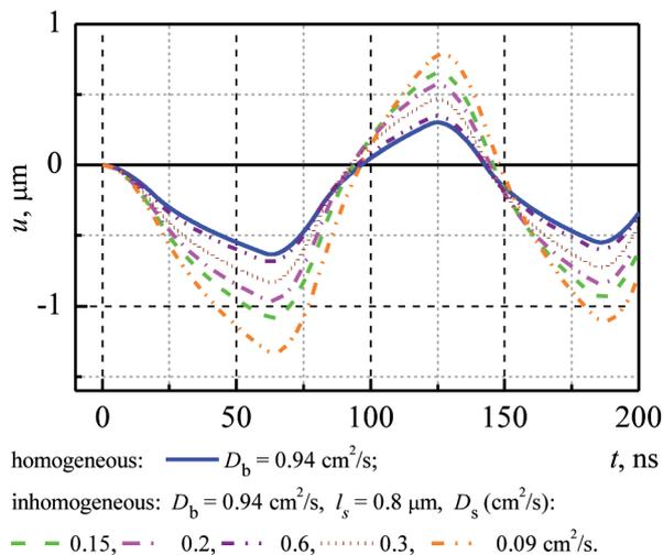
Fig. 6. Surface displacement evolution inhomogeneous (b) model two layer structures with different thermal diffusivity coefficient of top layer
