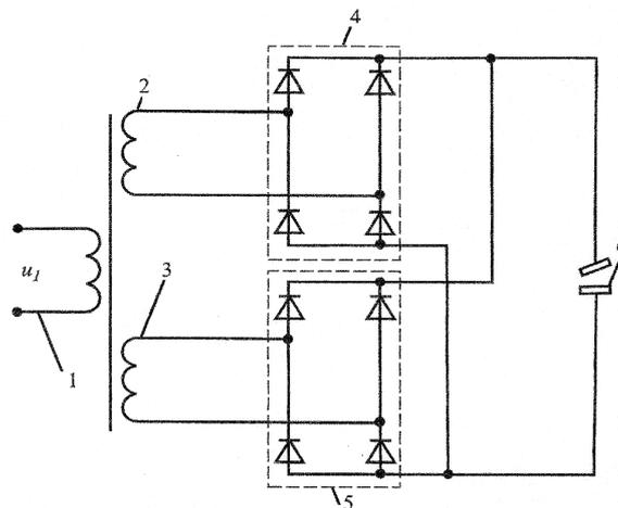
Fig. 1. Electric circuit of the double-bridge welding rectifier
