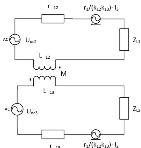
Fig. 4. Equivalent circuit of three-winding transformer
