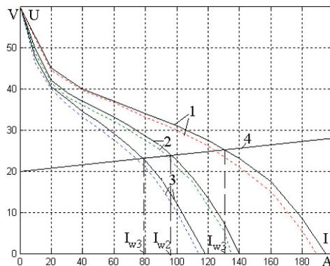
Fig. 7. The influence of the coupling factor for the leakage fluxes on the operating current of the rectifier: the curve 1 is for  $k = -0.3$ , the curve 2 is for  $k = 0$ , the curve 3 is for  $k = 0.3$ , and the curve 4 is the volt-ampere characteristics of a welding arc (1)
