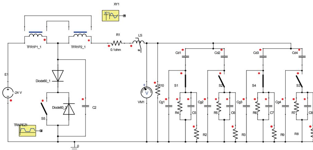
Fig. 2. Simulation model of pulsed power supply and a DBD reactor model
