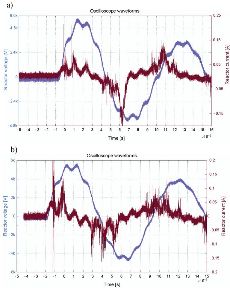
Fig. 7. Recorded oscilloscope waveforms in case of a) no additional inductance, b) saturable inductor
