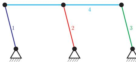
Fig. 3. A geometrically overconstrained double 4-bar mechanism
