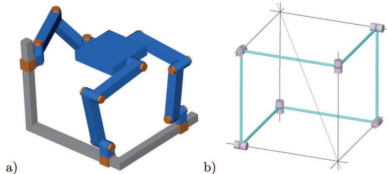
Fig. 2. a) An overconstrained parallel manipulator, b) The geometrically overconstrained Bricard mechanism
