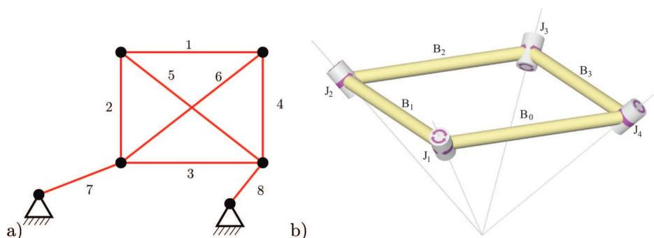
Fig. 1. a) A topologically overconstrained planar mechanism, b) A geometrically overconstrained spherical mechanism
