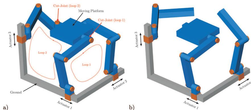
Fig. 7. a) Independent fundamental loops for the  $3\underline{P}RRR$  PKM. b) Tree-topology MBS model with 10 generalized coordinates
