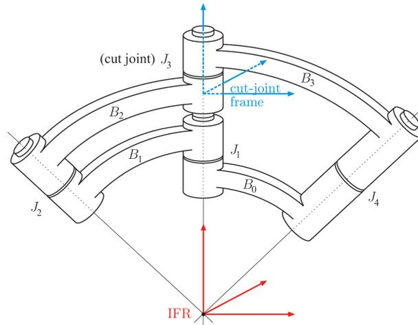
Fig. 6. Cut-joint and reference frame for spherical 4-bar mechanism. Shown is the reference configuration
