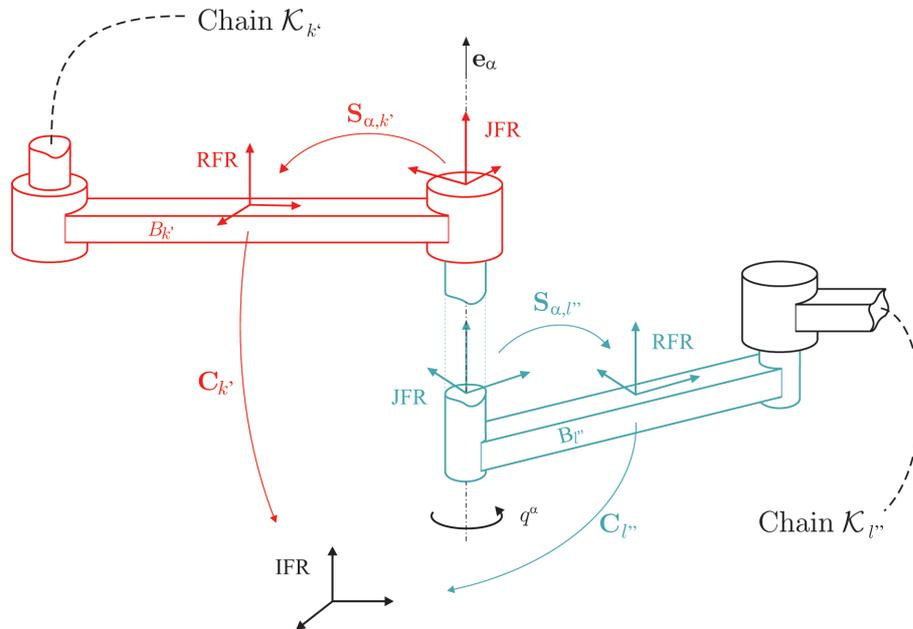
Fig. 5. Cut-joint kinematics
