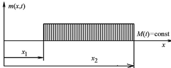
Figure 1. Model of actuator acting on the surface area (for example piezoceramics).
