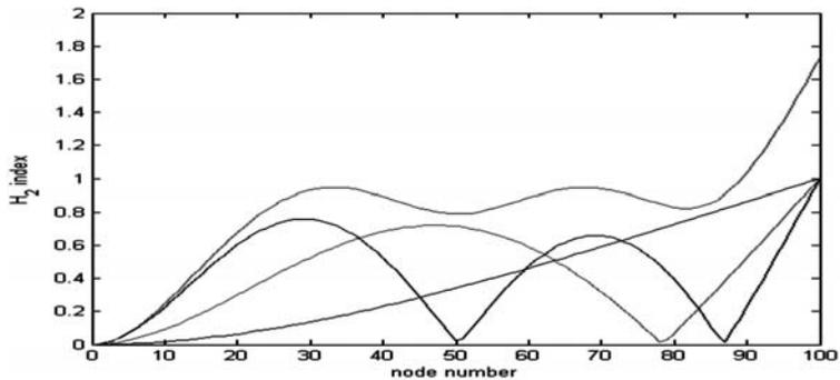
Figure 9. Evaluation of the first, second and third mode shapes simultaneously.
