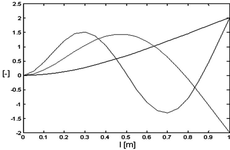
Figure 4. The first three mode shapes for the cases 2 and 4.
