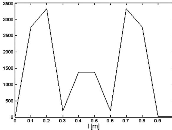
Figure 6. Performance index for the first three mode shapes.
