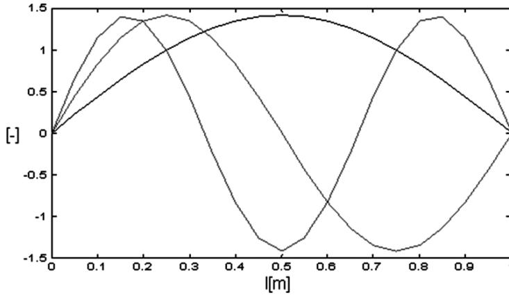
Figure 2. The first three mode shapes for the cases 1 and 3.
