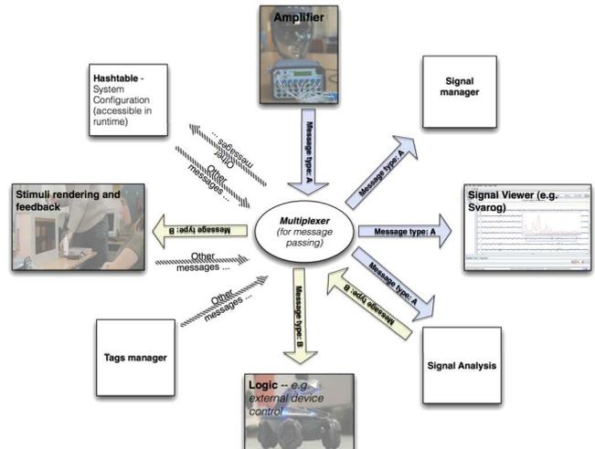
Fig. 4. General scheme of communication between OpenBCI modules
