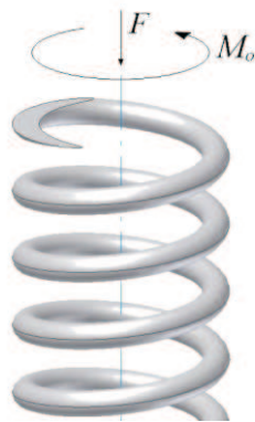
Fig. 2. Loads on segment of compressed spring
