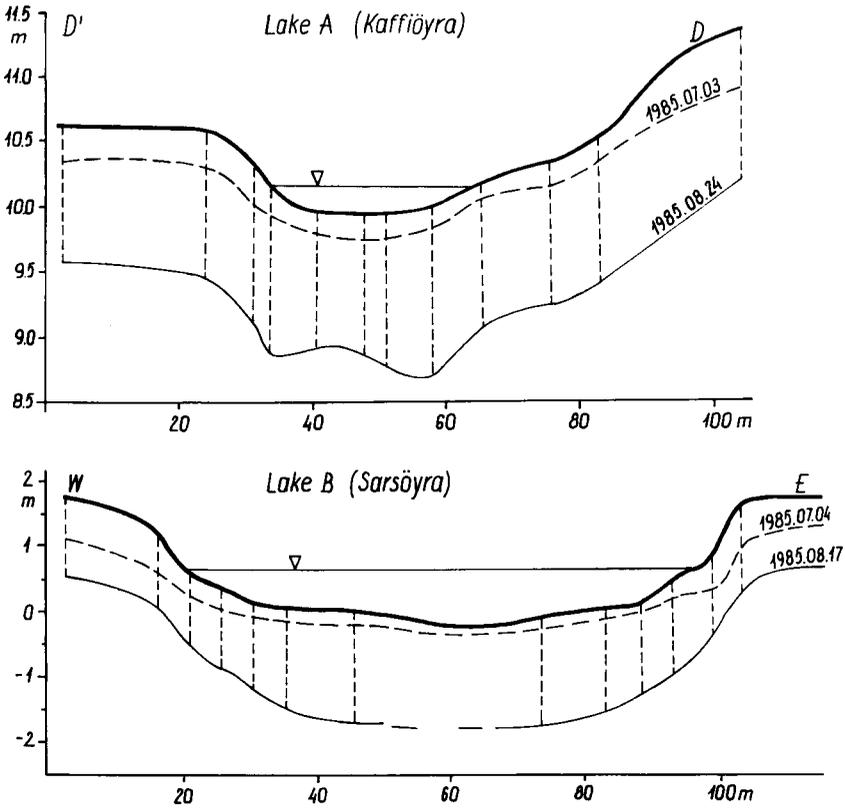
Fig. 5. Depth of soil thawing under and around the lakes A and B on presented days (cf. Fig. 2)
