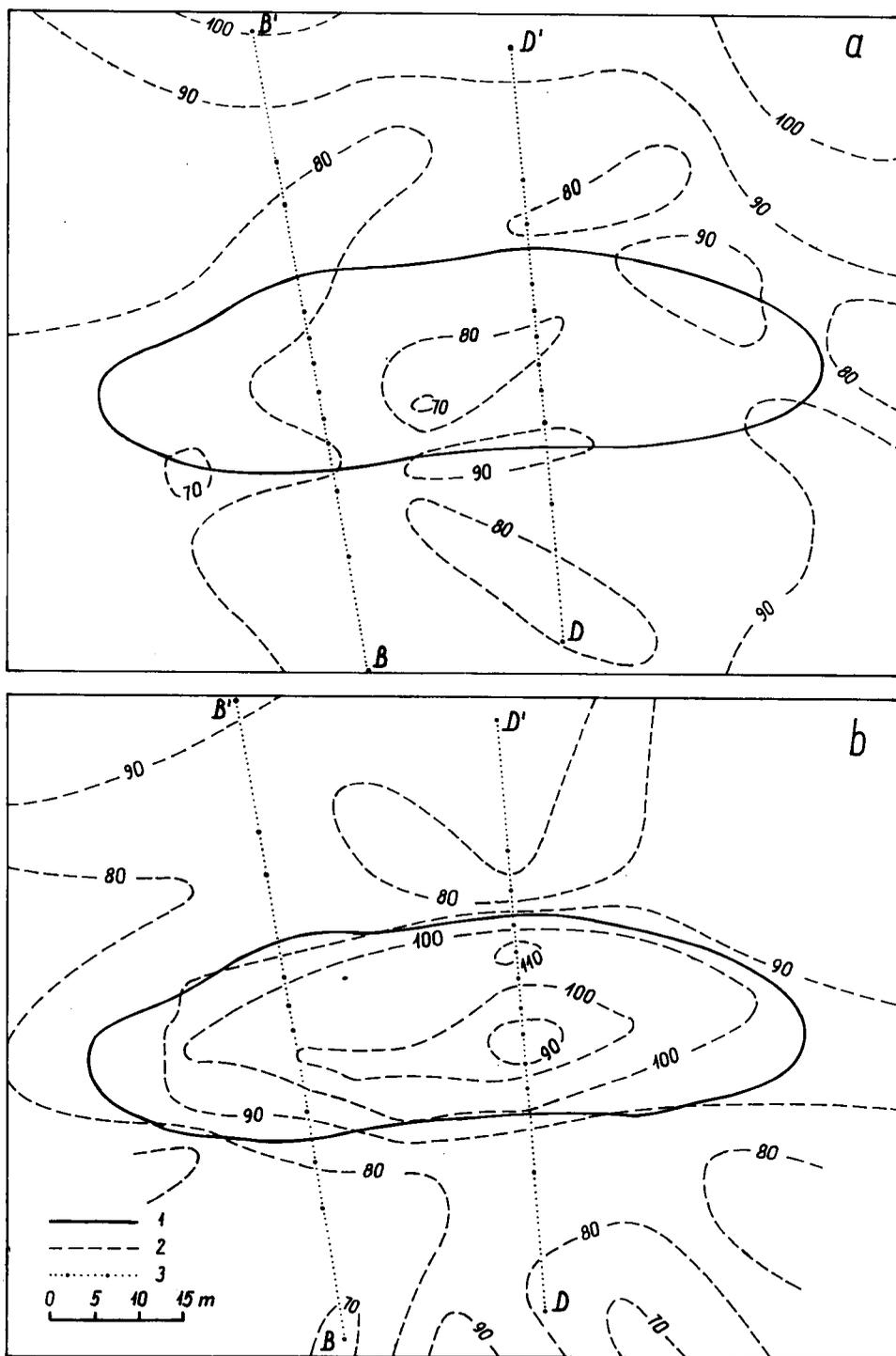
Fig. 4. Spatial variation of active layer under and around the lake A in 1982 on: a — August 21, b — September 6; 1 — shoreline, 2 — thickness of active layer in cm, 3 — measurement sections (cf. Fig. 2)
