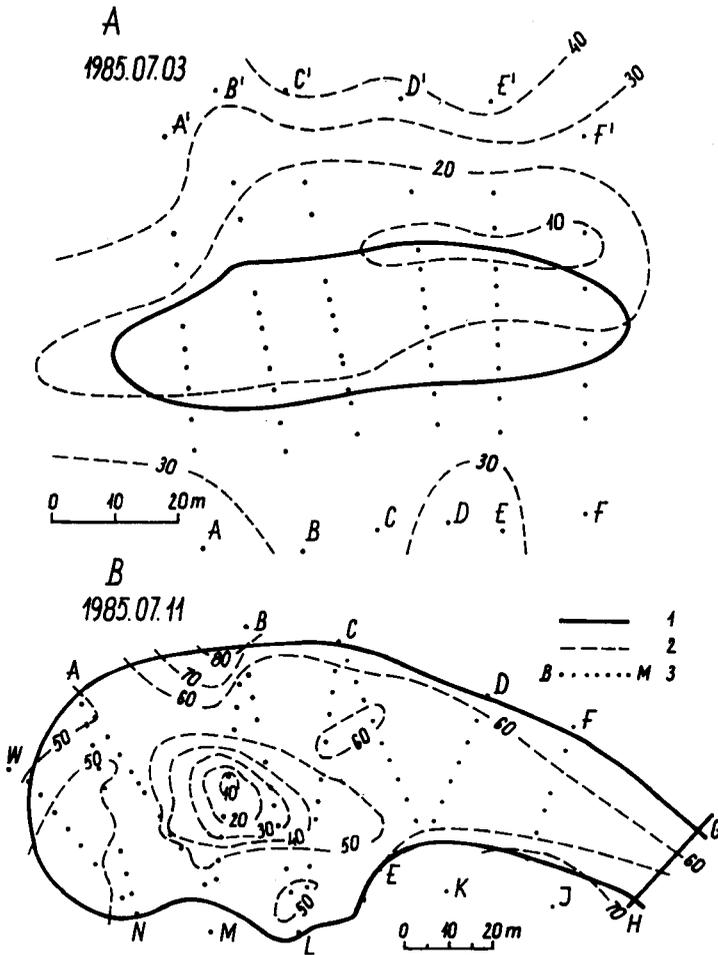
Fig. 6. Spatial variation of active layer thickness under and around the lakes A and B: 1 — shoreline, 2 — thickness of active layer in cm, 3 — measurement sections
