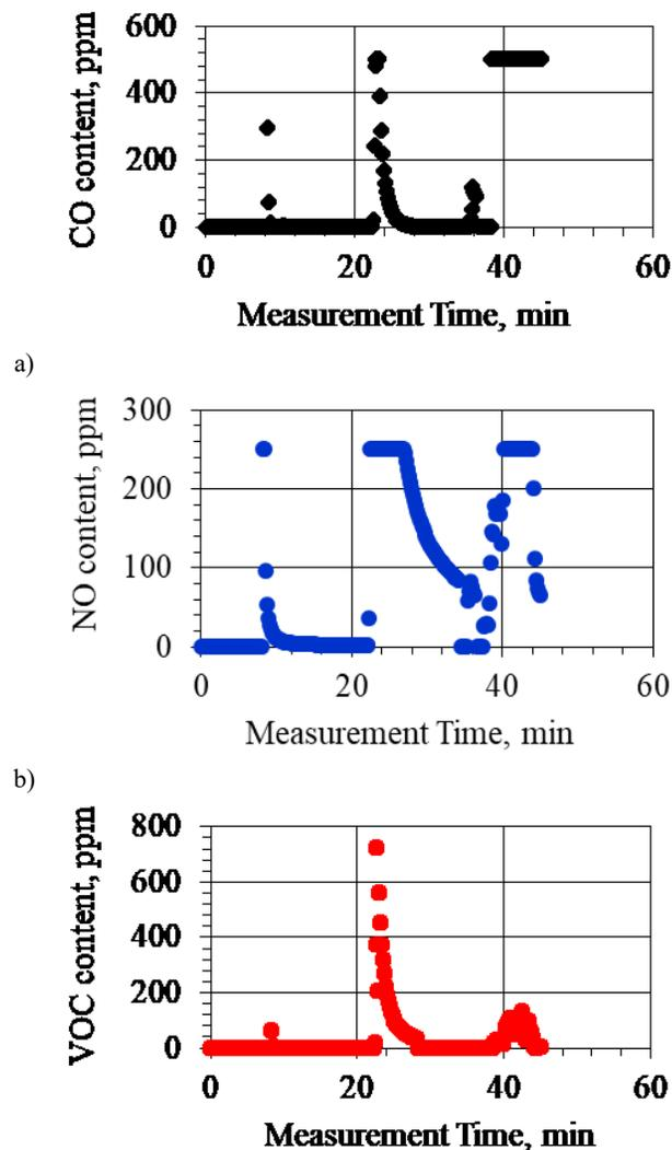
c) Fig. 3. a,b and c are analysis of gases emissions during reduction processes using Carbo-N-Ox reactants
