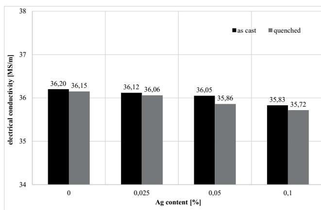
Fig. 2. Ag content (in the range 0,025mas. % to 0,1%mas) effect on the ambient temperature electrical conductivity of Al-Ag alloys. Materials prepared from commercial purity aluminium used for electrical applications
