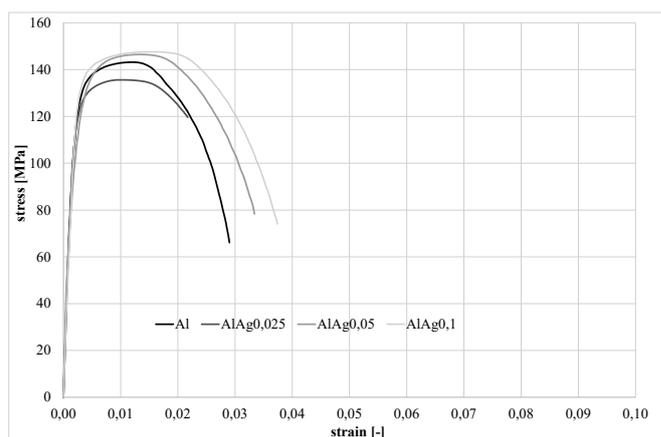
Fig. 4. Tensile tests of the Al and Al-Ag alloy wires after cold drawing (total strain 91%)
