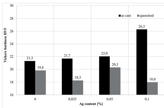
Fig. 3. Vickers hardness of Al-Ag alloys (with Ag content up to 0,1%mas.) in different tempers
