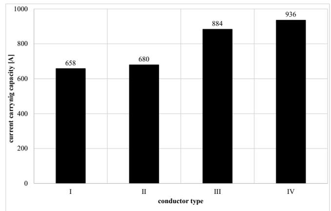
Fig. 10. Current carrying capacity of conductors from tab. 1 for maximum operating temperature; ambient temperature 293K ( $20^{\circ}\text{C}$ ), wind velocity 0,5m/s, solar radiation  $900\text{W}/\text{m}^2$
