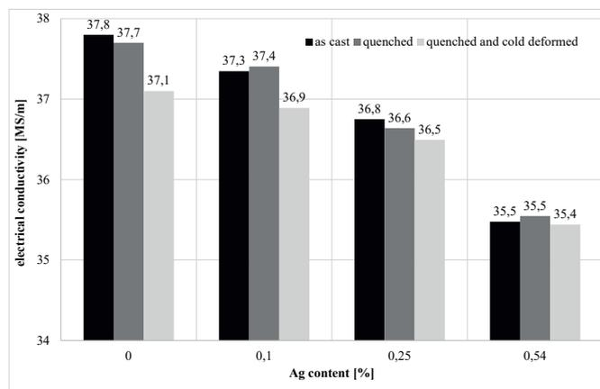
Fig. 1. Ag content effect on the ambient temperature electrical conductivity of Al-Ag alloys. Materials prepared from 99,99%mas purity base metals
