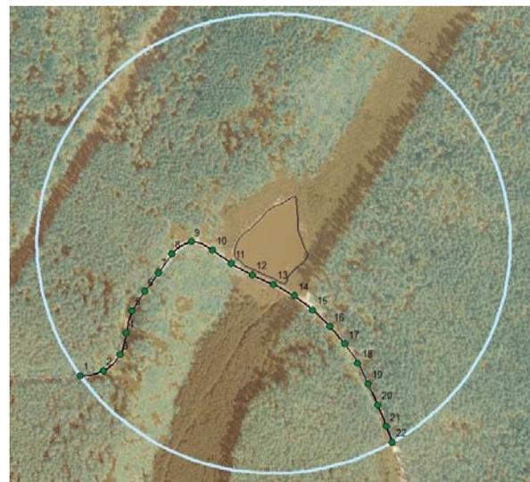
Fig. 3. A diagram of the adopted points along the road centre line on the orthophotomap base and on the basis of a Digital Surface Model; source: own elaboration
