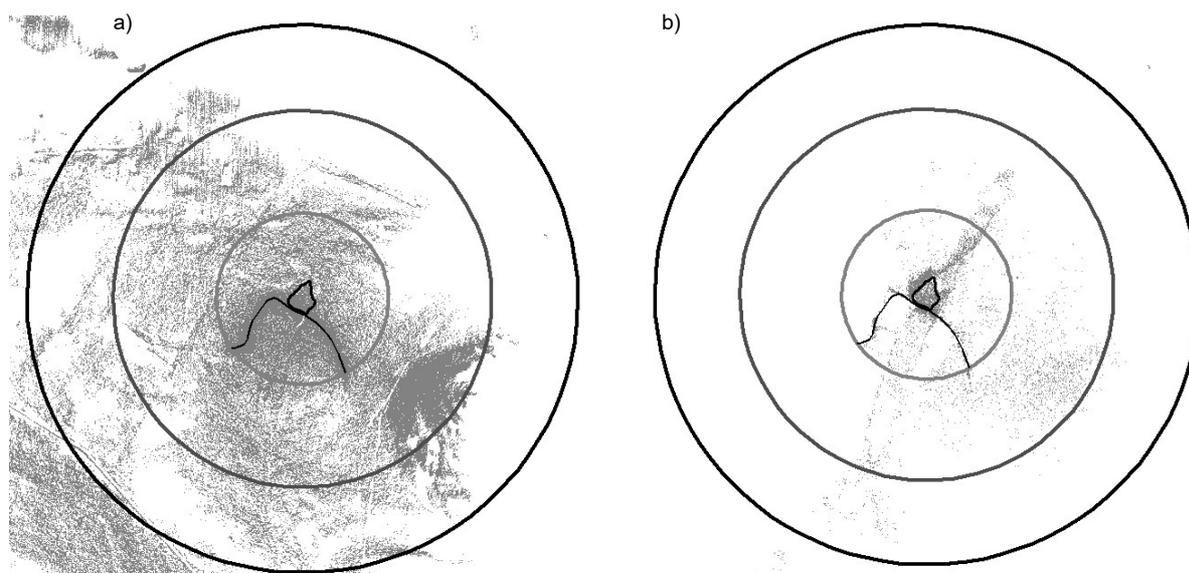
Fig. 5. The results of the visibility analysis within the range of 3 buffers: a) the results established on the basis of Digital Terrain Model, b) the effect of the Digital Surface Model application; grey colour represents visible areas, the remaining areas are invisible; source: own elaboration
