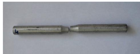
b) sample after fatigue test
