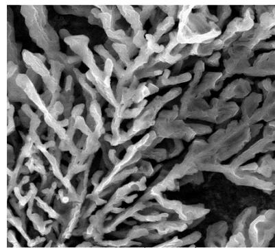
c) detail of rod-shape of silicon, etch. HCl, REM
