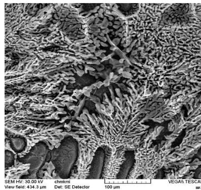
b) rod-shape of silicon, etch. HCl, REM
