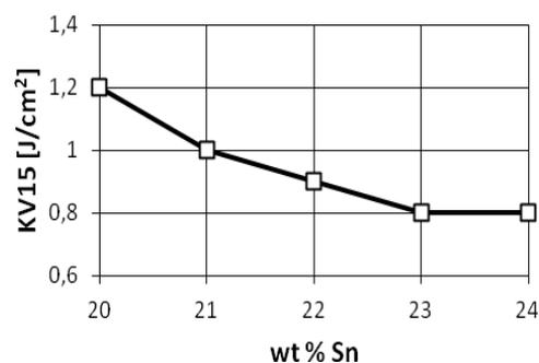
Fig. 4. Impact strength of high-tin bronzes versus tin content that there occurred full repeatability of impact strength test results
