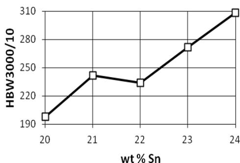
Fig. 2. Hardness of high-tin bronzes versus tin content
