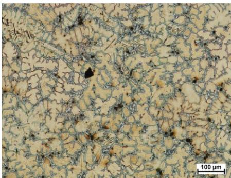
Fig. 6. Microstructure of alloy containing 20 wt% Sn
