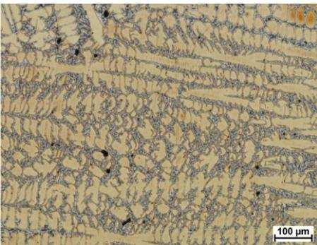
Fig. 8. Microstructure of alloy containing 22 wt% Sn
