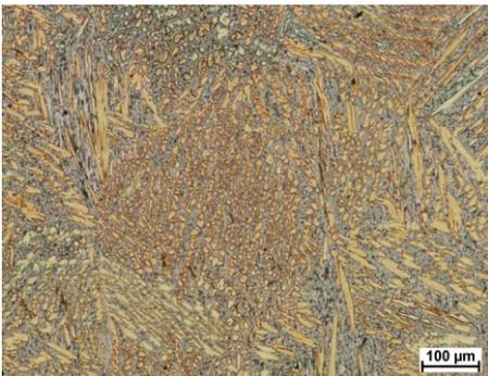
Fig. 9. Microstructure of alloy containing 23 wt% Sn
