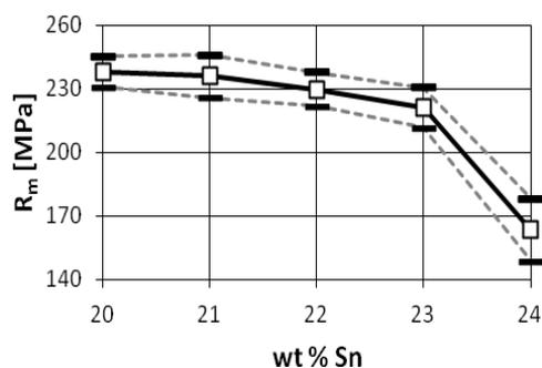
Fig. 1. Tensile strength  $R_m$  of high-tin bronzes versus tin content
