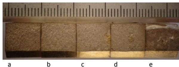
Fig. 5. Fractures of impact test specimens of various tin content: a) 20% Sn, b) 21% Sn, c) 22% Sn, d) 23% Sn, e) 24% Sn
