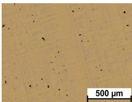
Fig. 3. Porosity of high-tin bronze specimen, 22 wt% Sn
