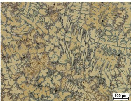
Fig. 7. Microstructure of alloy containing 21 wt% Sn
