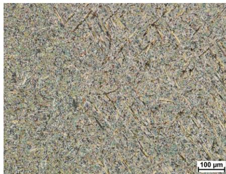
Fig. 10. Microstructure of alloy containing 24 wt% Sn
