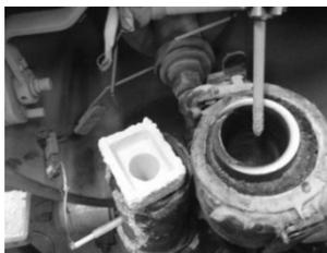
Fig. 2. Ceramic mould in a furnace chamber
