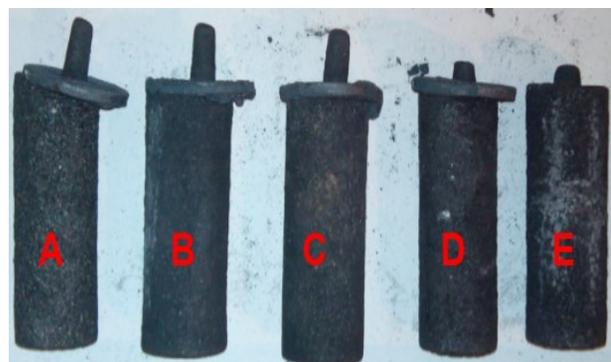
Fig. 3. Collected samples for test: Slag suspension without copper in the graphite crucibles (A, B, C, D, E - Preparations added to the process to remove the copper)
